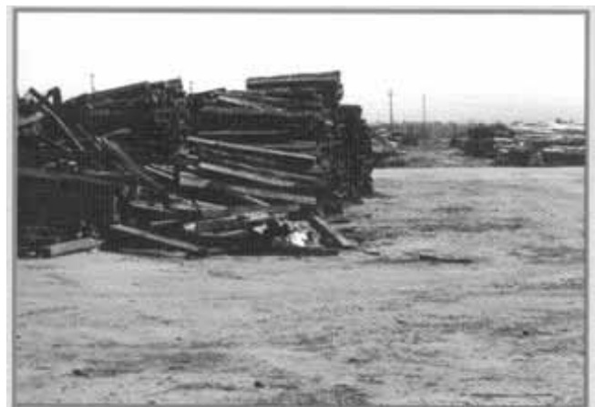
Railroad ties and logs for fuel at Wheelabrator Shasta Energy Company, Anderson, California. The power plant is allowed to burn not more than 25 percent railroad ties; burning plywood, particleboard, or plastic laminates is not permitted.
